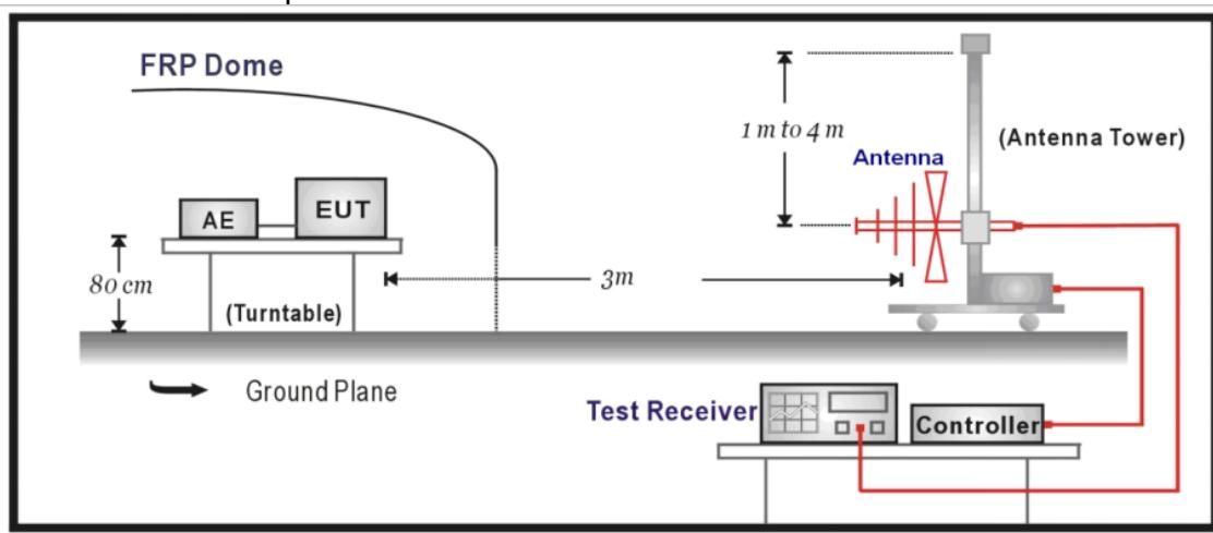
1GHz -40GHz Test Setup:
