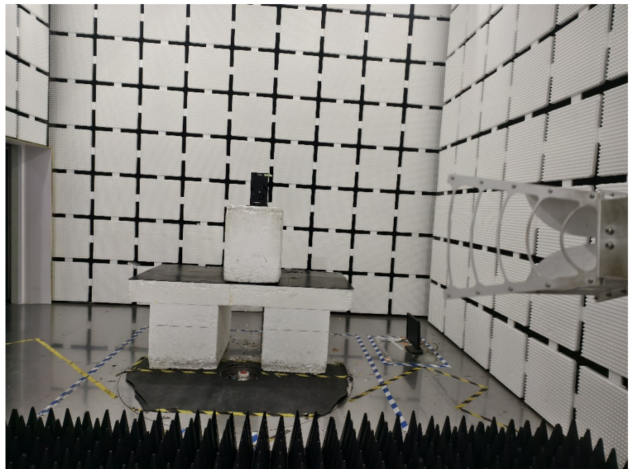
Radiation Emission Test Setup (1GHz to 18GHz)
