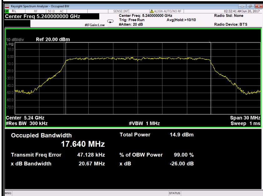
**Antenna 1****IEEE 802.11n HT 20 MHz mode / 5180 ~ 5240MHz****26dB Bandwidth (CH Low)**
