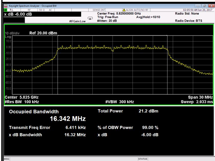
**Antenna 1****IEEE 802.11a mode / 5745 ~ 5825MHz****6dB Bandwidth (CH Low)**
