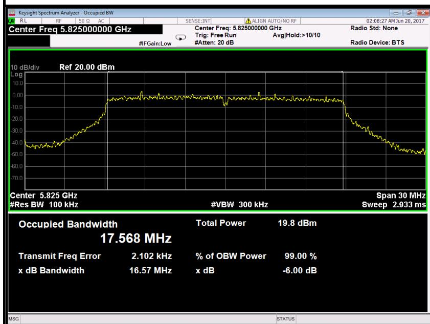
**Antenna 1****IEEE 802.11n HT 20 MHz mode / 5745 ~ 5825MHz****6dB Bandwidth (CH Low)**
