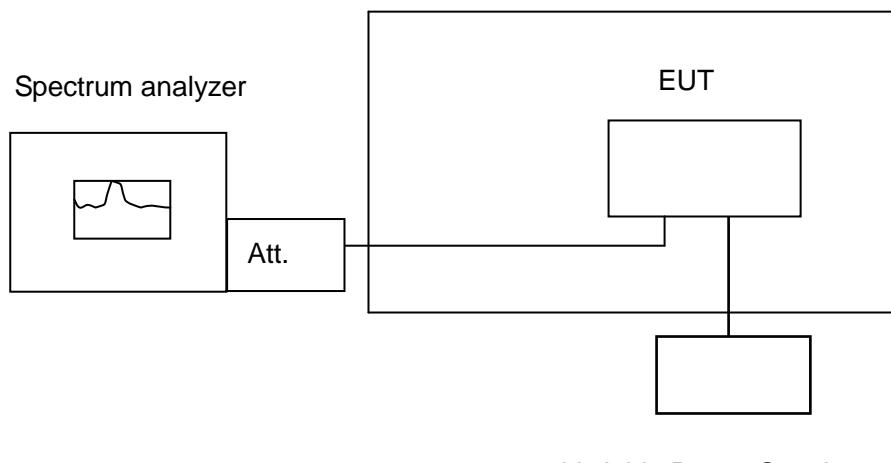
**Remark:** Measurement setup for testing on Antenna connector
