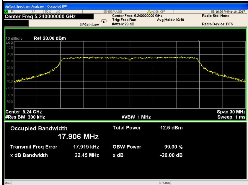
**Antenna 1****IEEE 802.11n HT 20 MHz mode / 5180 ~ 5240MHz****26dB Bandwidth (CH Low)**
