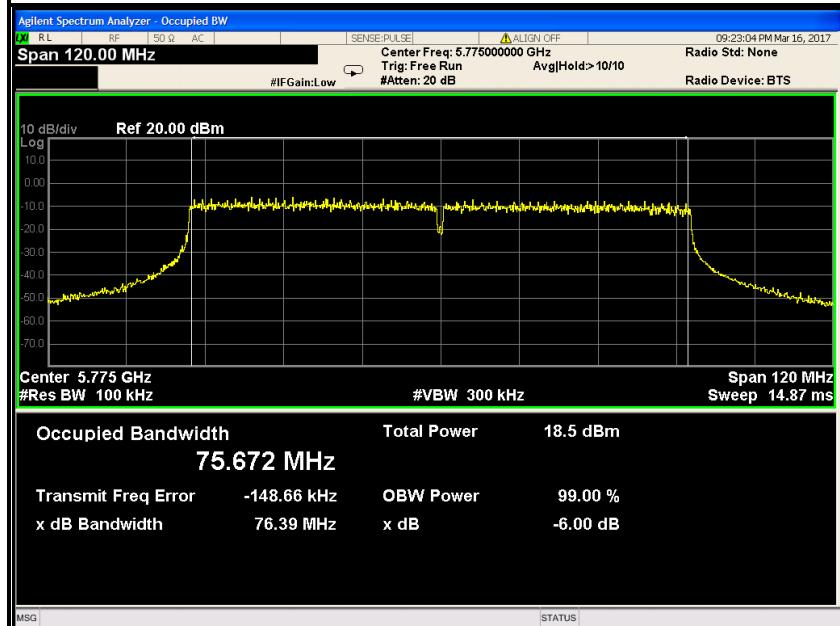
**Antenna 1****IEEE 802.11ac 80 mode / 5775MHz****6dB Bandwidth**
