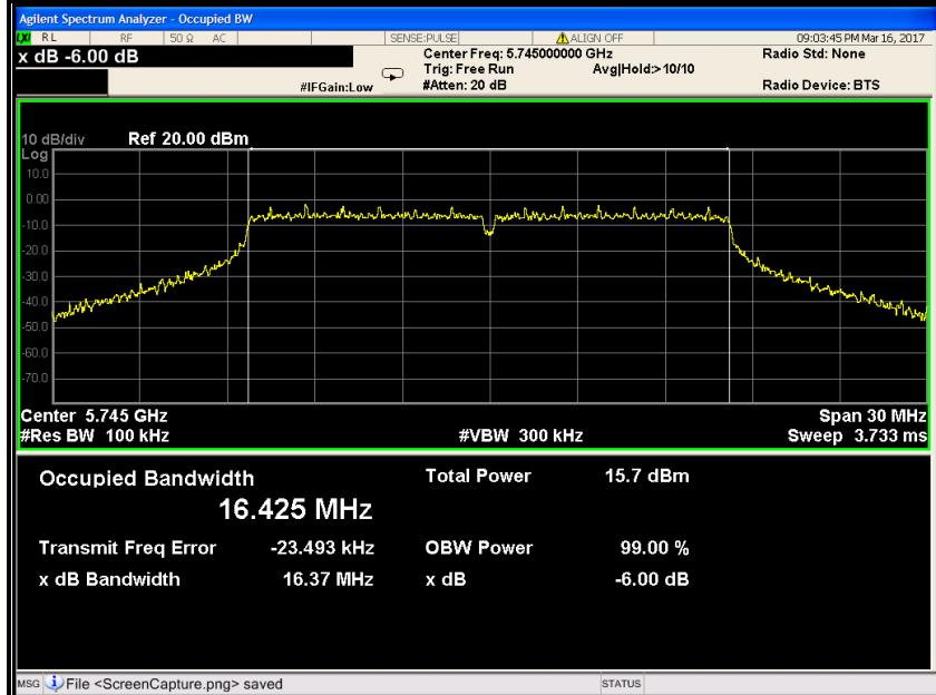
**6dB Bandwidth (CH Mid)**
