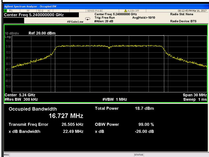
**Antenna 1****IEEE 802.11a mode / 5180 ~ 5240MHz****26dB Bandwidth (CH Low)**
