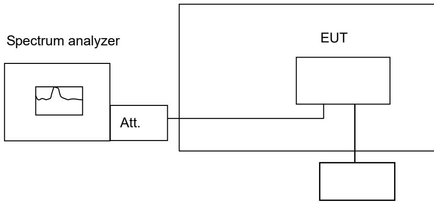
**Remark:** Measurement setup for testing on Antenna connector
