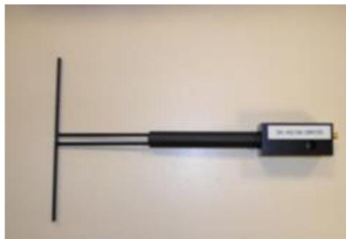
Figure 1 – Satimo COMOSAR Validation Dipole
