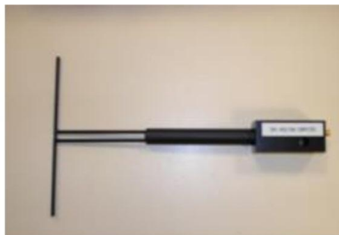
Figure 1 – Satimo COMOSAR Validation Dipole
