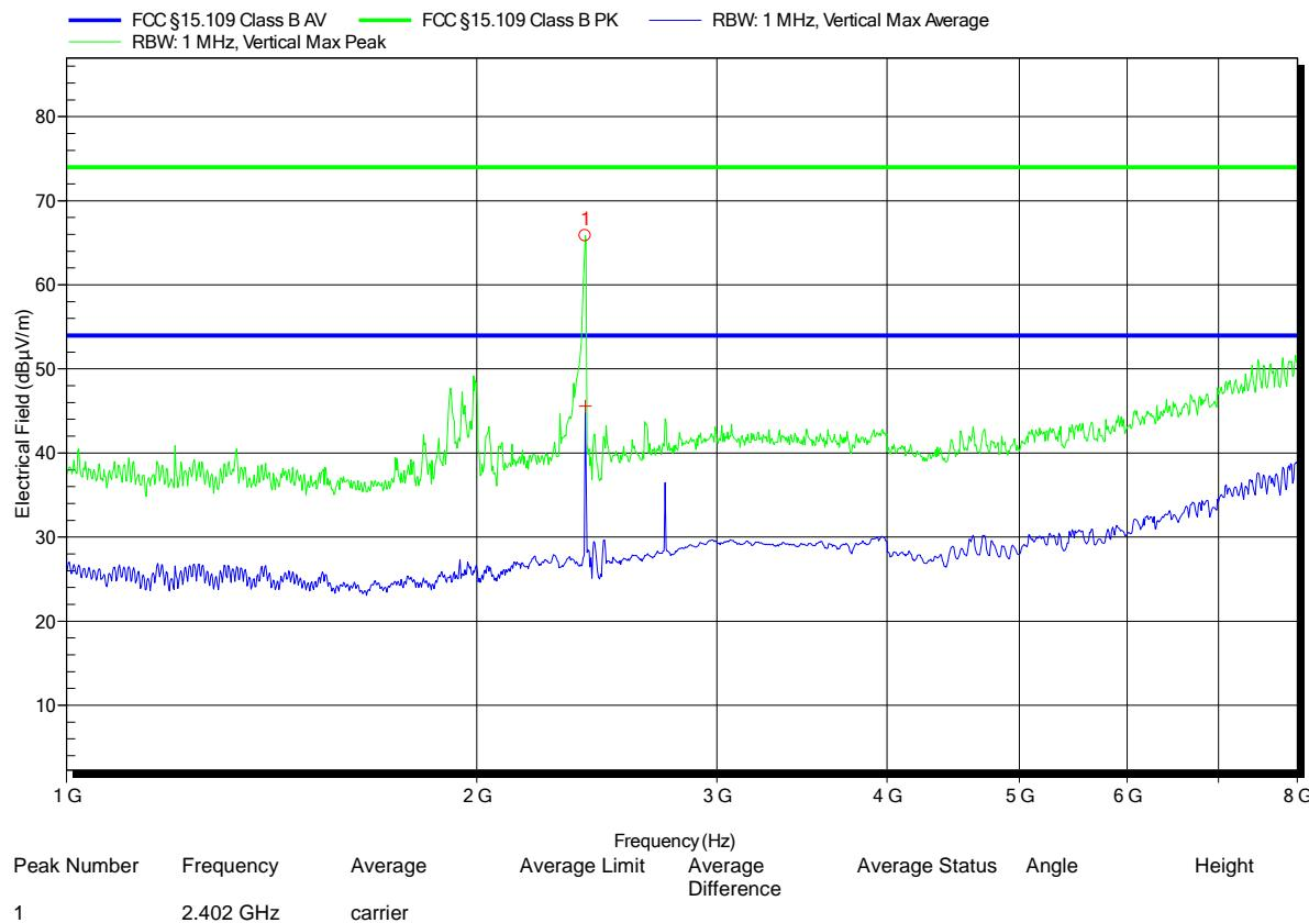
**Spurious emissions under normal conditions according to FCC Part 15b**
