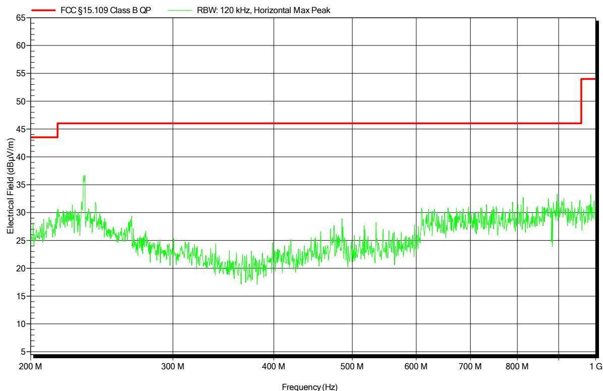
**Spurious emissions under normal conditions according to FCC Part 15b**
