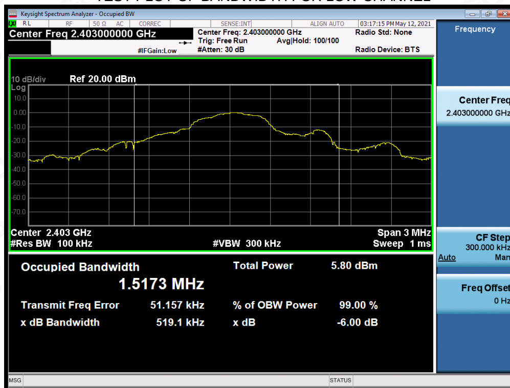
TEST PLOT OF BANDWIDTH FOR LOW CHANNEL
