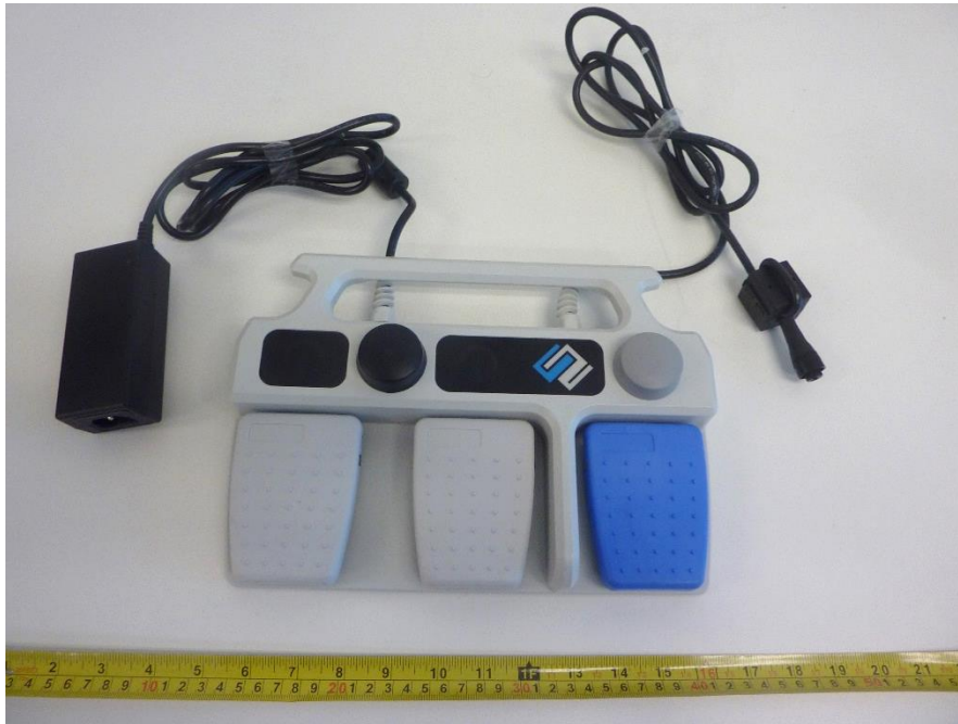
Figure 5: Foot Pedal Switch to provide 12VDC to controller
