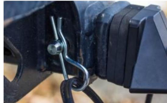
6. Connect the power cable with the connector on the vehicle.
