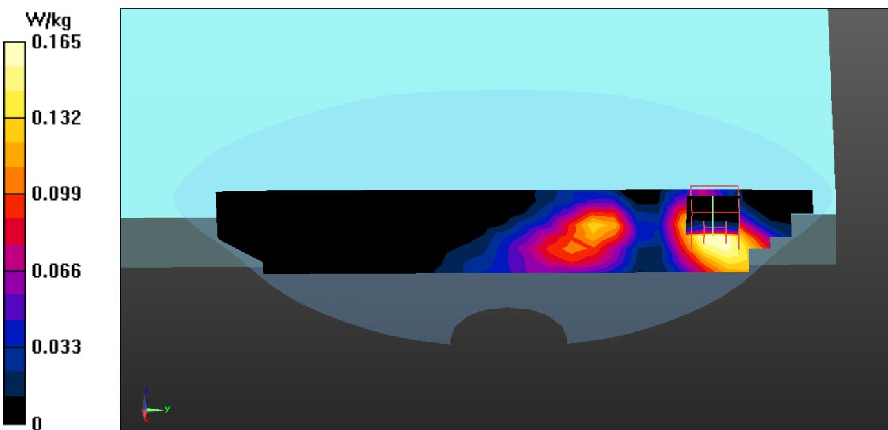
**802.11a EUT Bottom (Aux Antenna), Z-Axis plot****Channel: 157**
