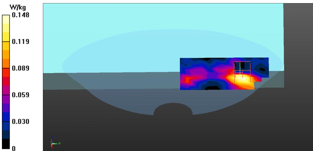
**802.11a EUT Bottom (Aux Antenna), Z-Axis plot**
