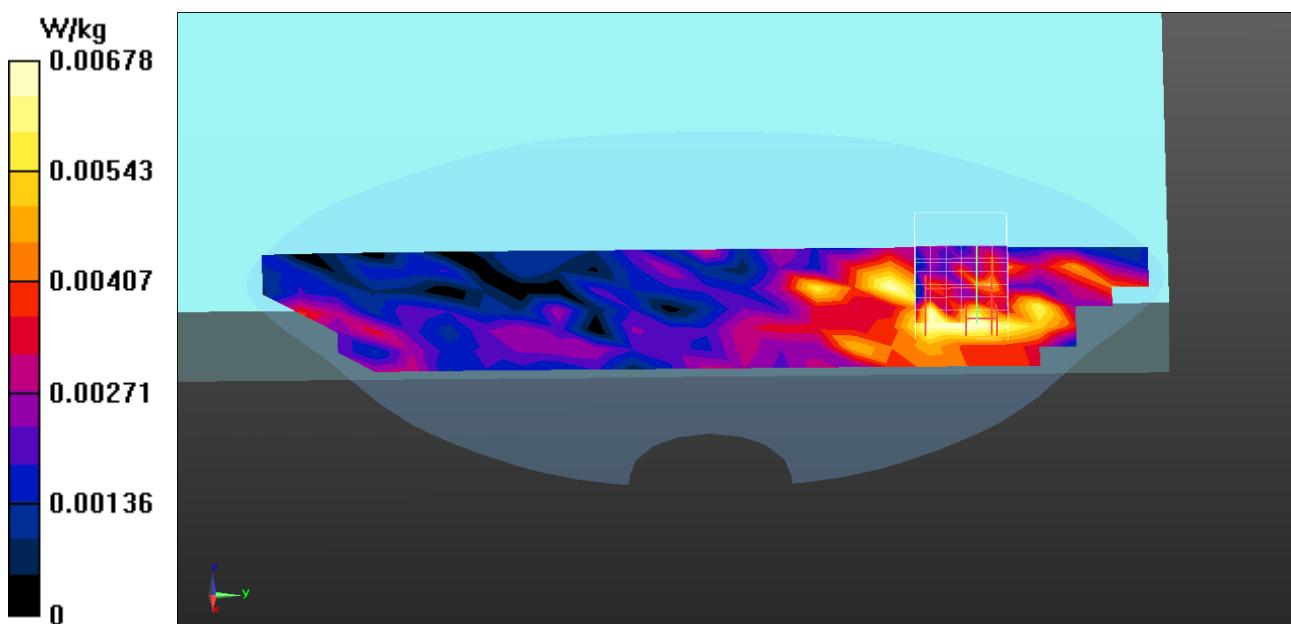
**802.11b EUT Bottom (Aux Antenna) Z-Axis plot**
