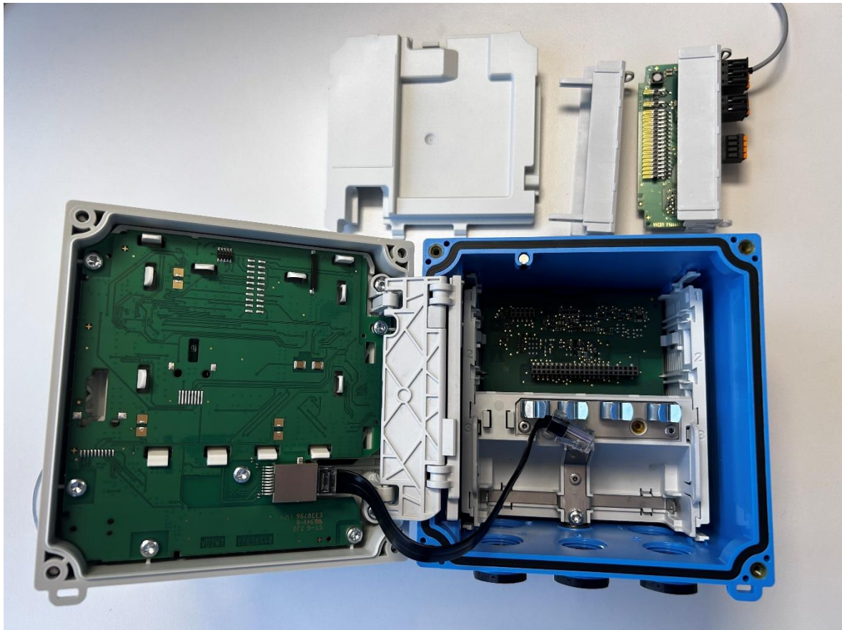
Figure 5 : View of the Opened Top Side – middle Module removed
