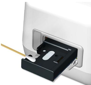
The blood, moisture or dust that enters the tray may lead to failure of the MARK-B™ 1 analyzer. Wipe the tray carefully with an alcohol-moistened swab if needed.
