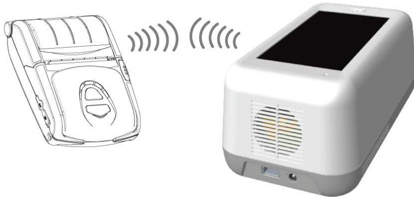
(2) First, turn on the Bluetooth in the Bluetooth Setting menu and select the printer to connect and pair with the analyzer.
