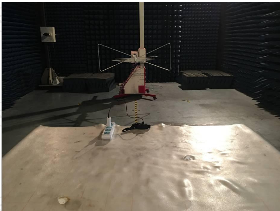
Radiated Emission Test View
