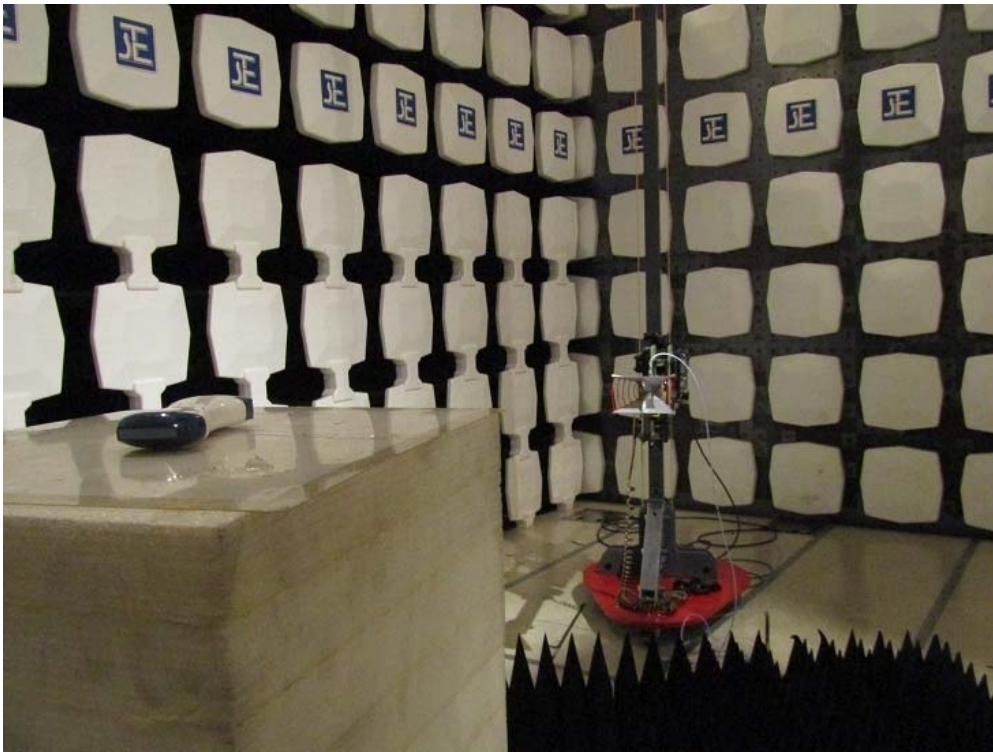
Measurement of Radiated Emission Test Set Up
