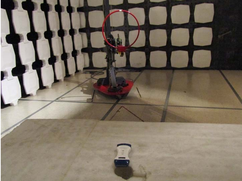
Measurement of Radiated Emission Test Set Up
