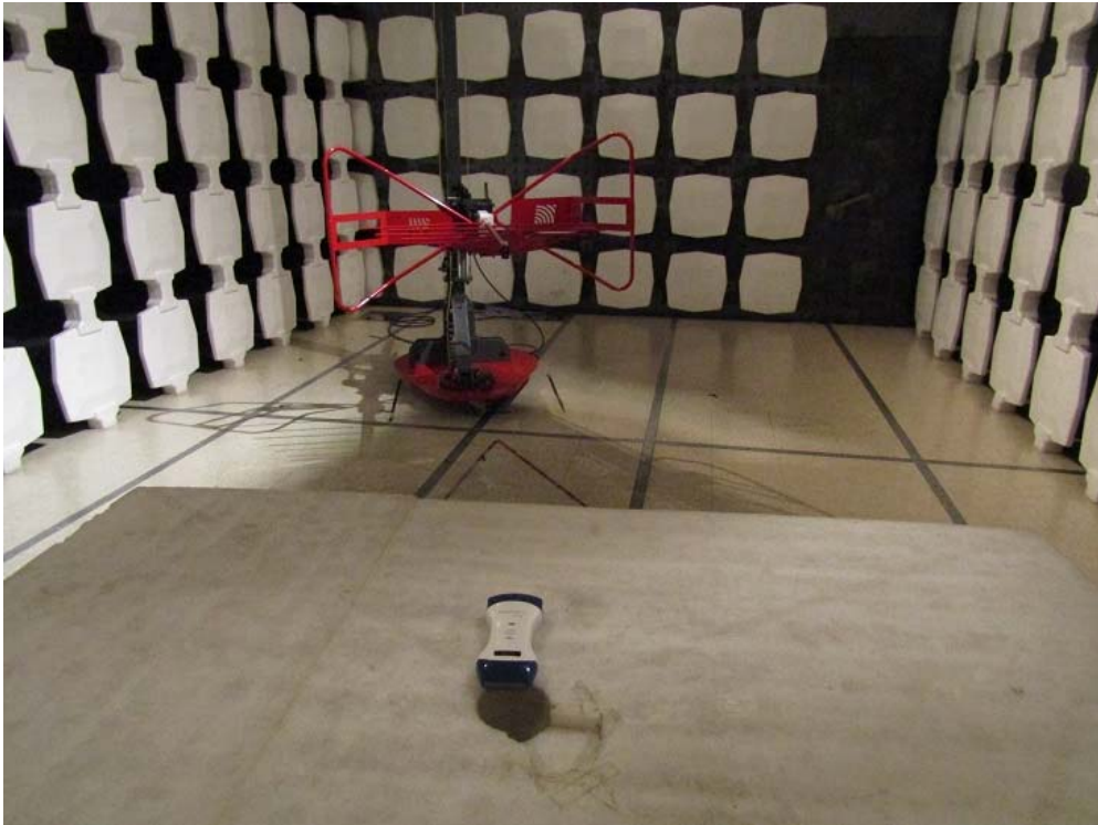
Measurement of Radiated Emission Test Set Up
