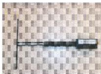
Figure 1 – Satimo COMOSAR Validation Dipole
