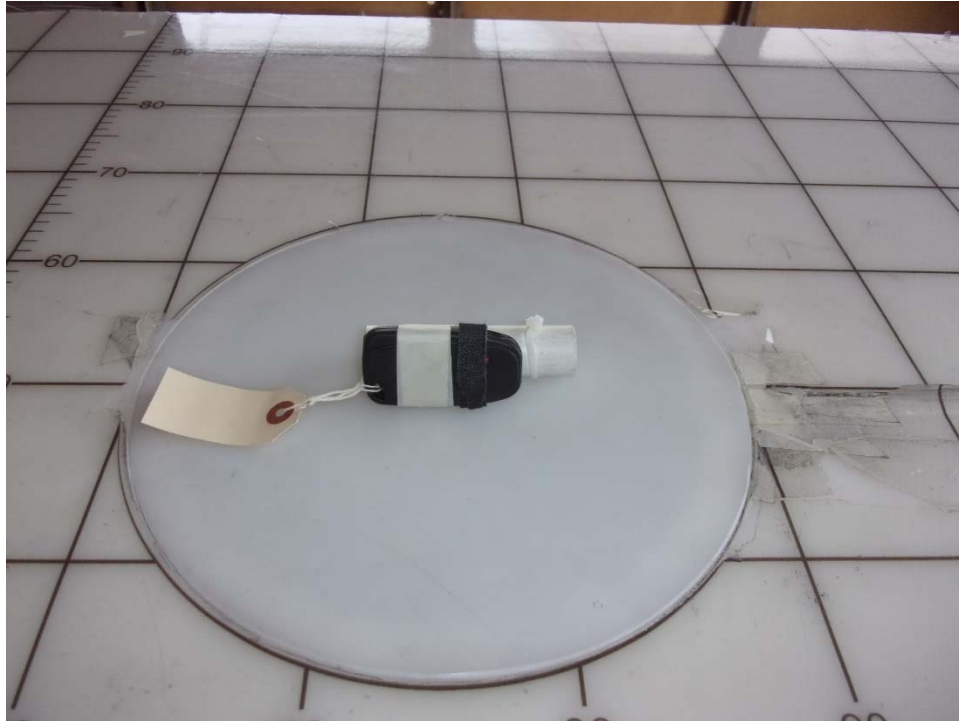
Test Setup, Z Axis, Below 1 GHz
