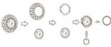
If you want to wear IVY as bracelet, the first thing to do is remove the necklace metal fitting and add bracelet metal fitting. Above picture shows how to do that. After putting the bracelet metal fitting, you can put the battery and close the back cover by hand or by tool.
