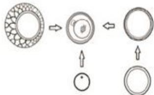
After IVY is open, put the battery where you see the battery contacts. Make sure the -ve side of battery is facing down and you can see the +ve side of the battery. After putting the battery, close the back cover either by hand or tool. Rotate clockwise to close.
