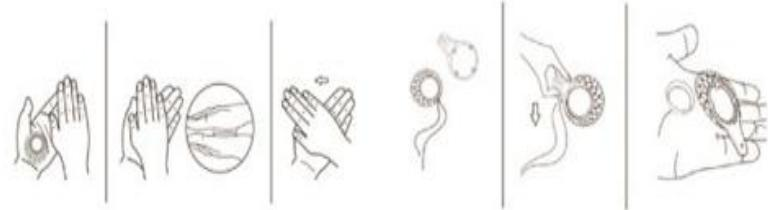
You have to open IVY to insert or replace battery, or to change from necklace to bracelet. The above picture shows how to open IVY using hand. Rotate anti-clockwise to open.
