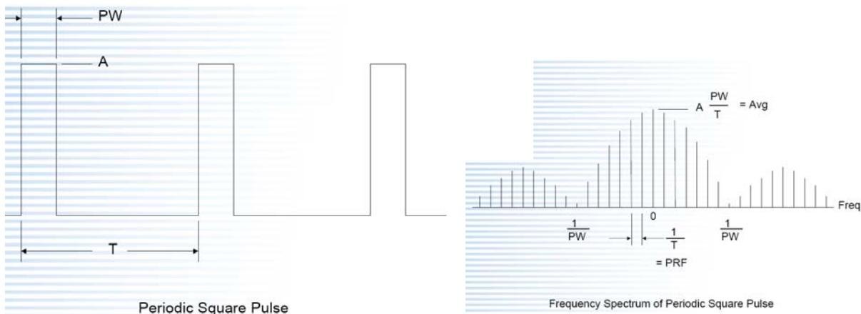
If using spectrum analyzer to measure pulse signal , it have to make sure the RBW use is at least 2/PW.
