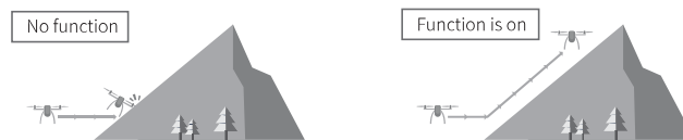
Schematic diagram of altitude aiding
