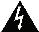
The lighting flash with arrowhead symbol, within an equilateral triangle, is intended to alert user to the presence of uninsulated "dangerous voltage" within the product's enclosure that may be of sufficient magnitude to constitute risk of electric shock to persons.
