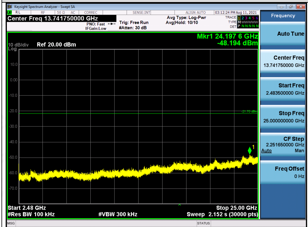
Test_Graph_802.11n20_ANT1_2437_MCS0_Higher Band Emissions
