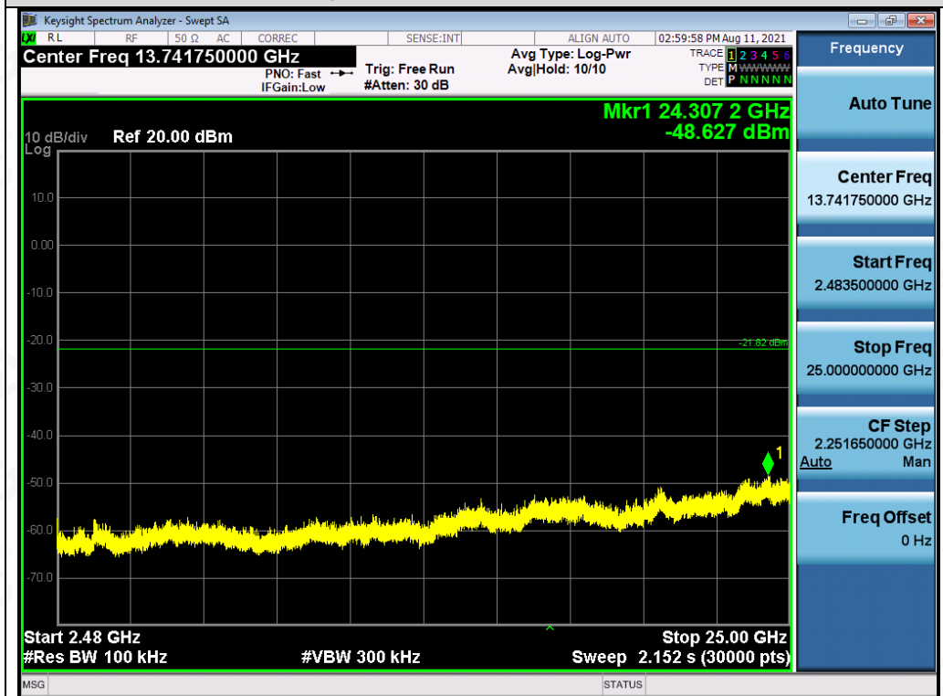
Test_Graph_802.11g_ANT1_2437_6Mbps_Higher Band Emissions
