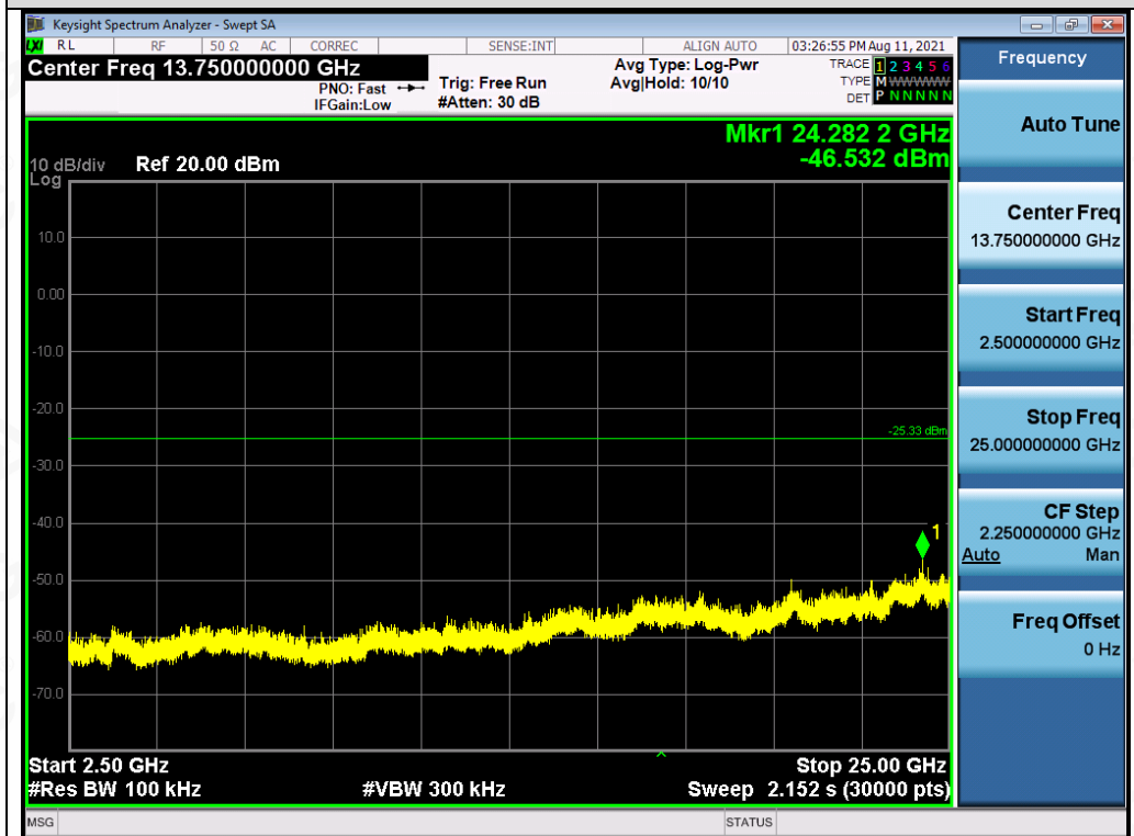
Test_Graph_802.11n40_ANT1_2452_MCS0_Higher Band Emissions
