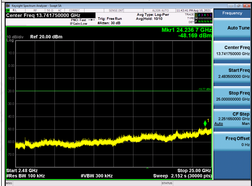
Test_Graph_802.11b_ANT1_2412_1Mbps_Higher Band Emissions
