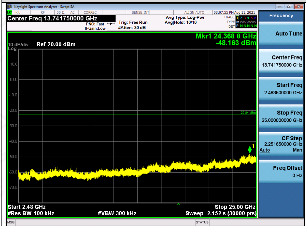
Test_Graph_802.11n20_ANT1_2412_MCS0_Higher Band Emissions
