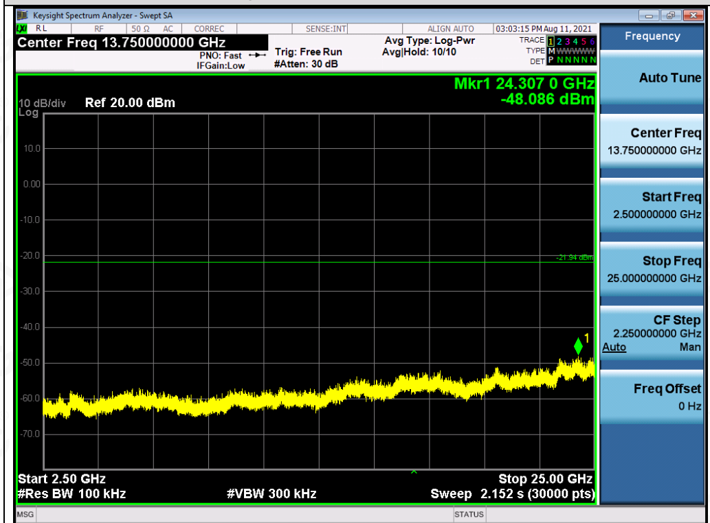
Test_Graph_802.11g_ANT1_2462_6Mbps_Higher Band Emissions
