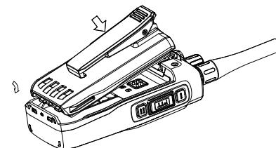
To install the battery □ fit in the battery to the battery compartment from the bottom of the battery. Press the top part of the battery towards the IP smart terminal until a click is heard. The battery is locked in place.
