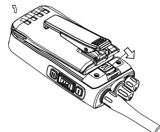
To remove the battery – power off the terminal, push the battery lock upwards subsequently pull the top part of the battery away from the IP smart terminal. Lift up the whole battery.
