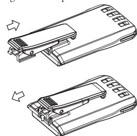
Align the grooves of the belt clip with those of the battery. Push the belt clip into the groove until it is latched on.
