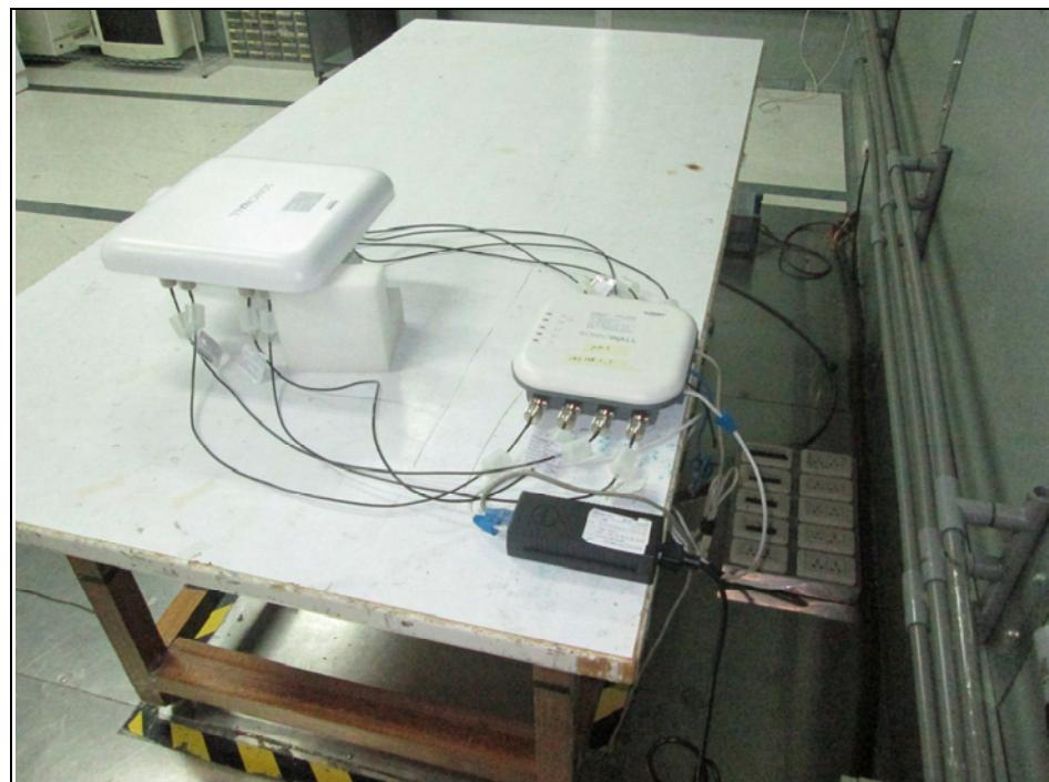
CONDUCTED EMISSION TEST (Test Mode F)
