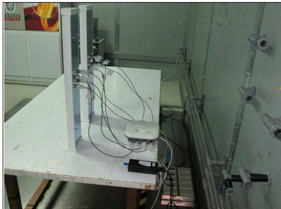
CONDUCTED EMISSION TEST (Test Mode C)
