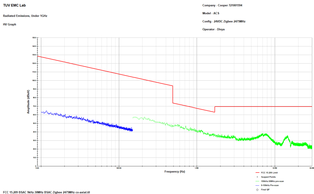
Figure 2.3.6-2: Radiated Spurious Emissions – 9 kHz – 30 MHz - HCH- 2475 MHz
