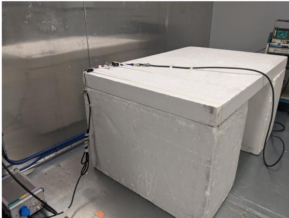
Figure 7: Test Setup – Conducted Emissions
