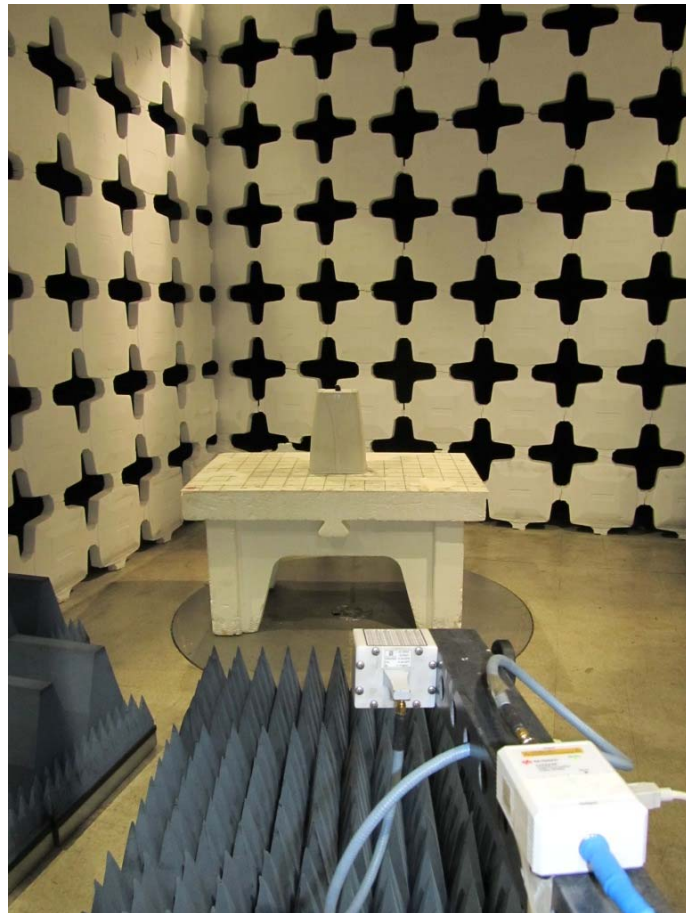
Photo 4. Radiated emissions test setup with Horn antenna in 18-25GHz.
