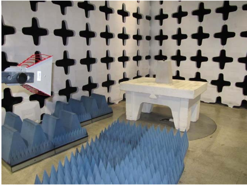
Photo 3. Radiated emissions test setup with Horn antenna in 1-18GHz.
