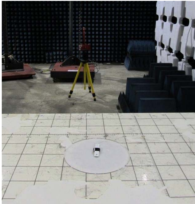
Photo 1.. Radiated emissions test setup with Loop antenna.
