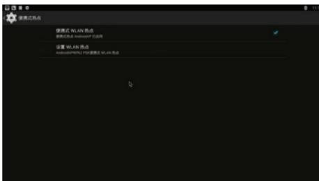
Select "Setup WLAN Hotspot" to set up "Network SSID", "Security", "Password" parameters
