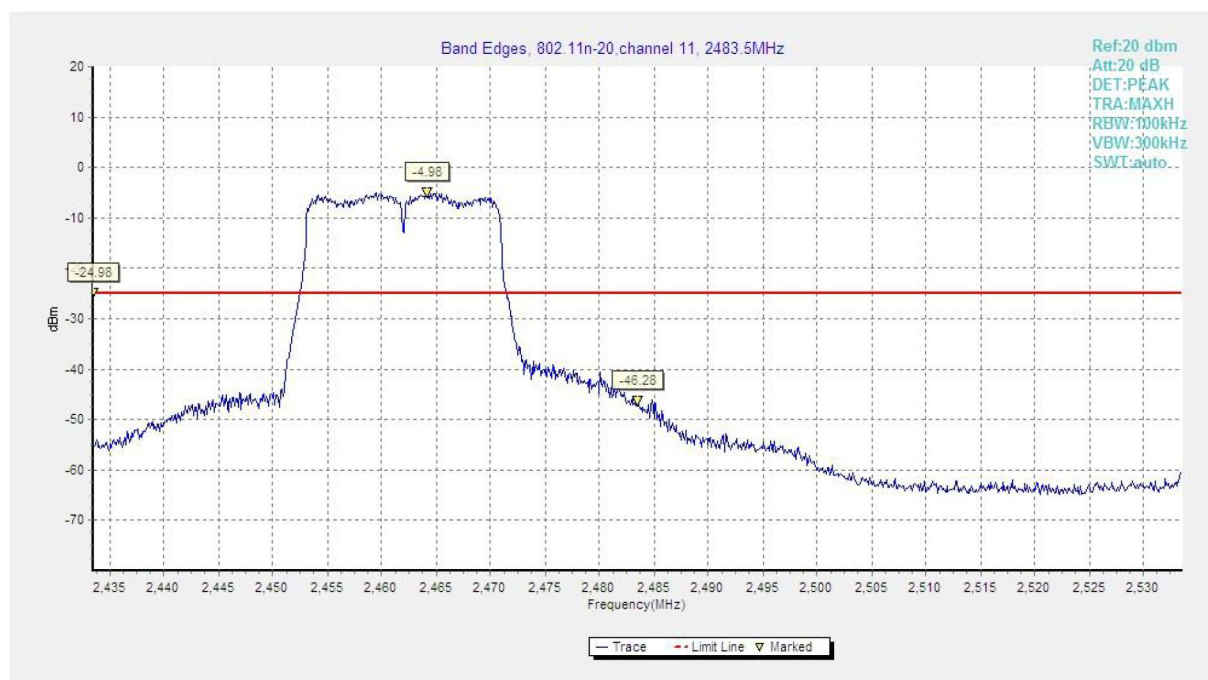
Fig.24 Band Edges (802.11n HT20, CH 11)
