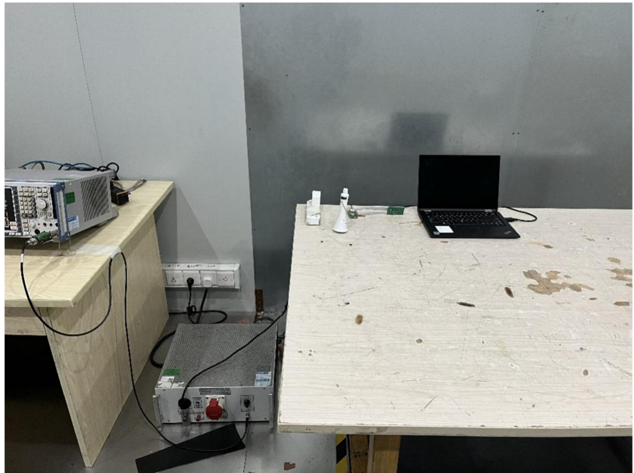
Conducted Emission Test Setup
