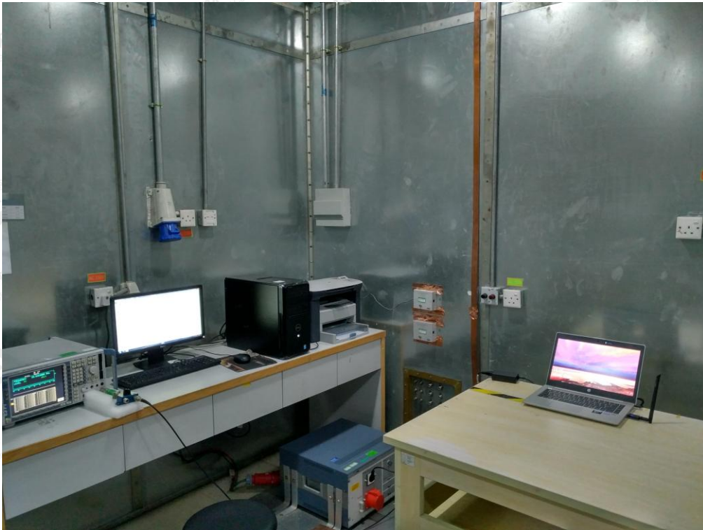
FCC RADIATED EMISSION TEST SETUP BELOW 1GHZ
