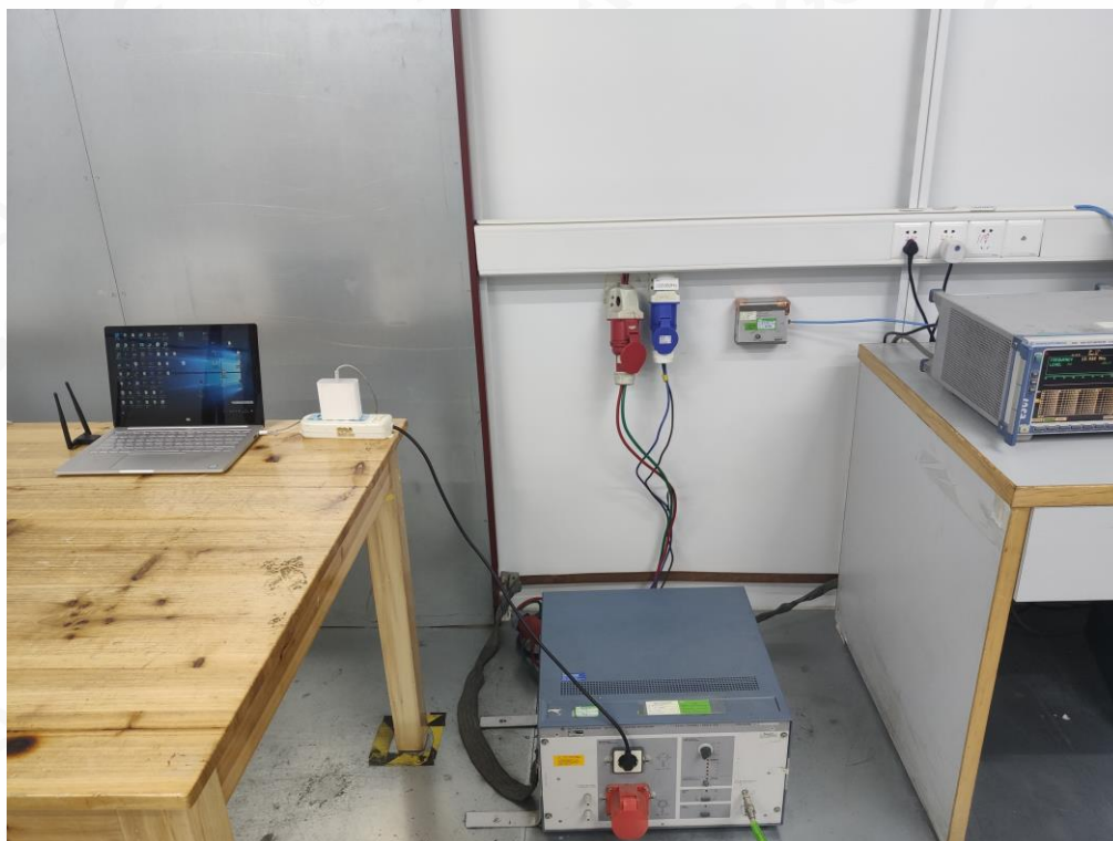
FCC RADIATED EMISSION TEST SETUP BELOW 1GHZ
