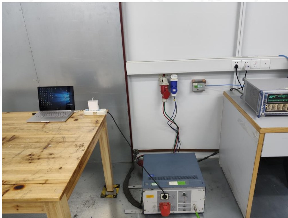
FCC RADIATED EMISSION TEST SETUP BELOW 1GHZ
