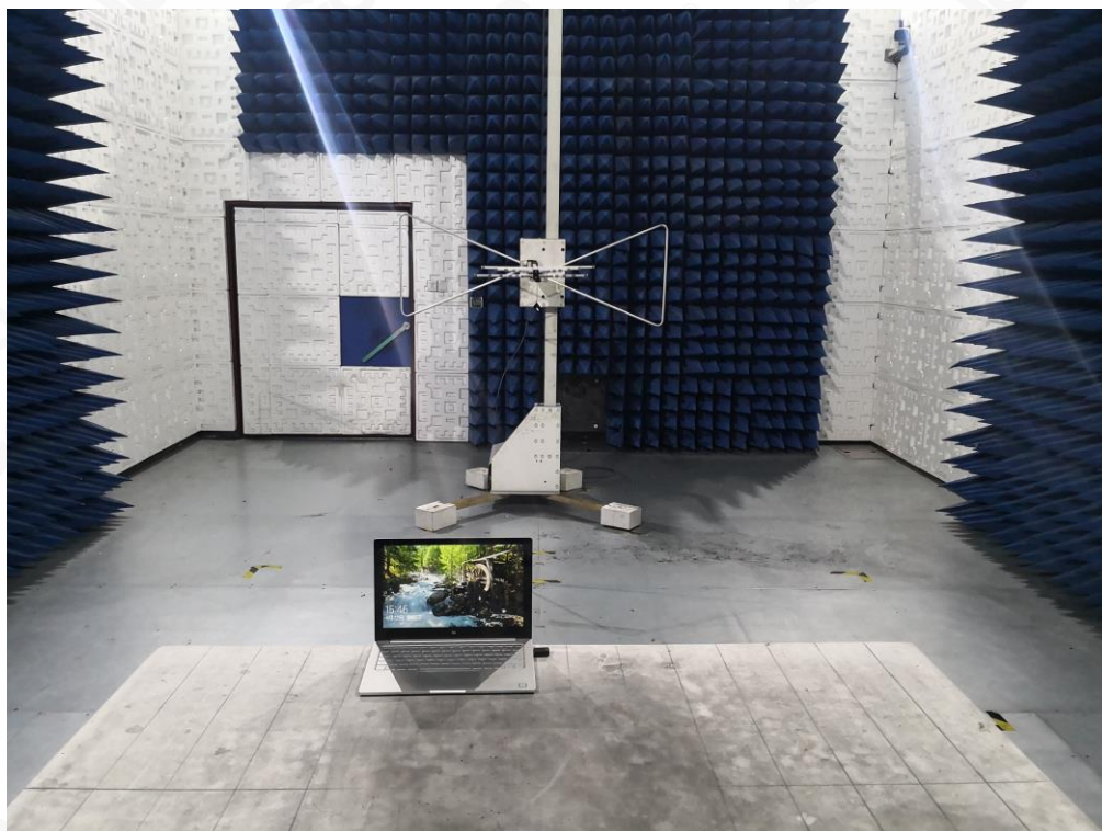
FCC RADIATED EMISSION TEST SETUP BELOW 1GHZ
