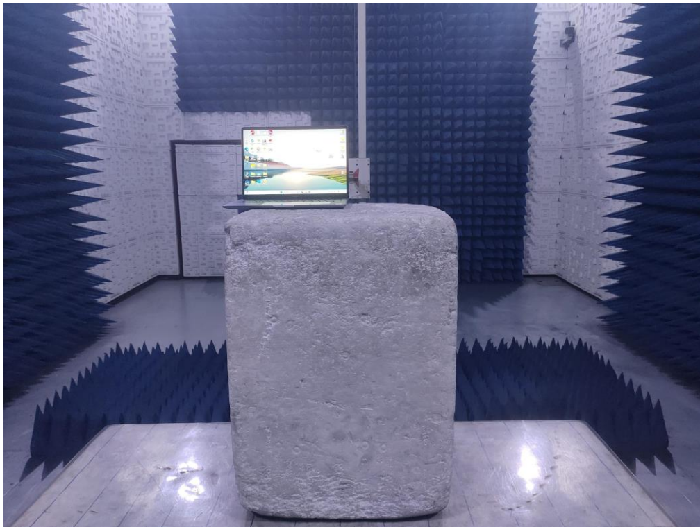
RADIATED EMISSION TEST SETUP ABOVE 1GHz
