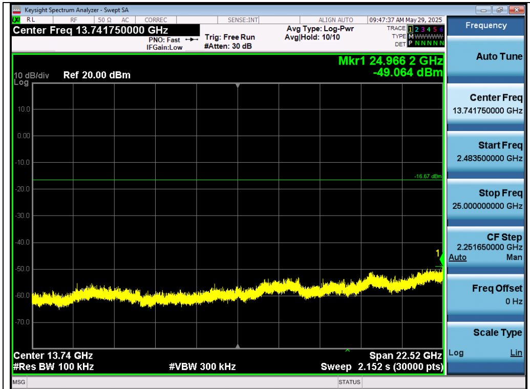
Test_Graph_BR_ANT1_2402_1Mbps_Higher Band Emissions
