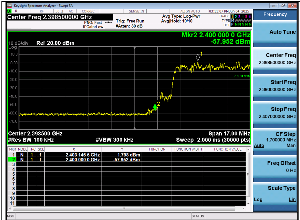
Test_Graph_EDR_HOP_ANT1_NA_3Mbps_Lower Band Edge Emissions
