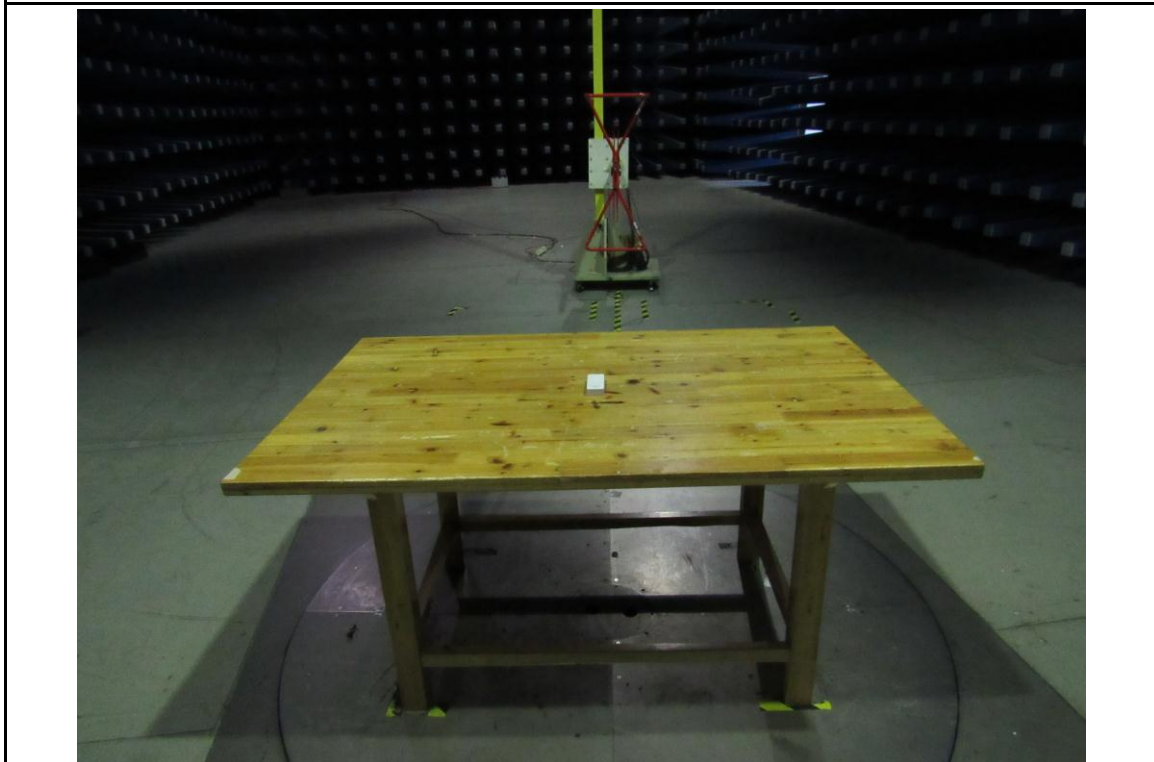
Radiated Emissions Test Setup Below 1GHz Rear View
