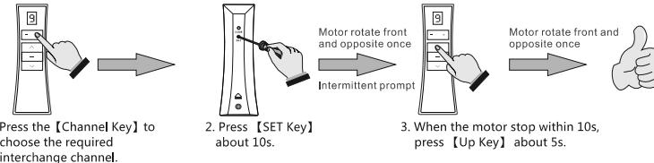
Up/Down limit setting: Up/Down limit means curtain run Up/run Down can reach high/low position. This function is only applicable to electronic limit function of the receiver(motor)
