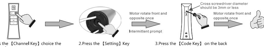
Channel copy: Increase another transmitter for the receiver(motor) which have been match the code, and receiver(motor) can be controlled by several transmitters
