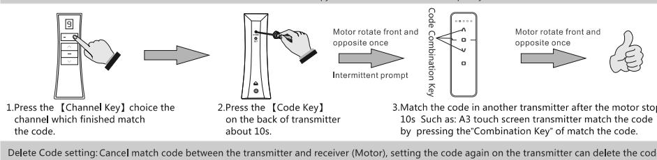
Delete Code setting: Cancel match code between the transmitter and receiver (Motor), setting the code again on the transmitter can delete the code.
