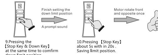
Note: If you want to reset the limit position Again operate Up/Down limit set up step.
