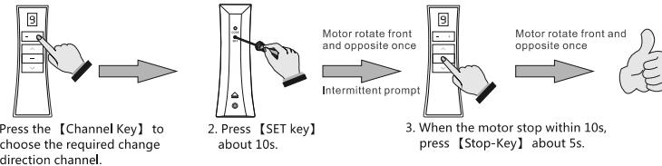
Inching/Continuous move mode change: Switch key function for the code setted receiver (motor), after the switch , receiver (motor) rotate little if you press the up or down key on the transmitter(N09-N16 without this function )
