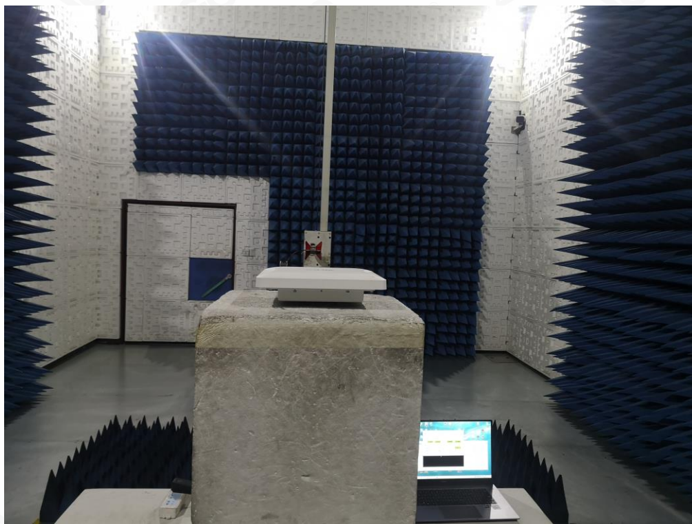
FCC RADIATED EMISSION TEST SETUP-ABOVE 1GHz
