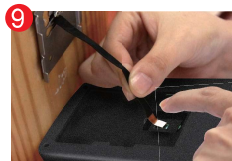
Connect cable socket to connection base.
