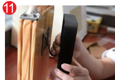
Protect cable before fixing emitter.
