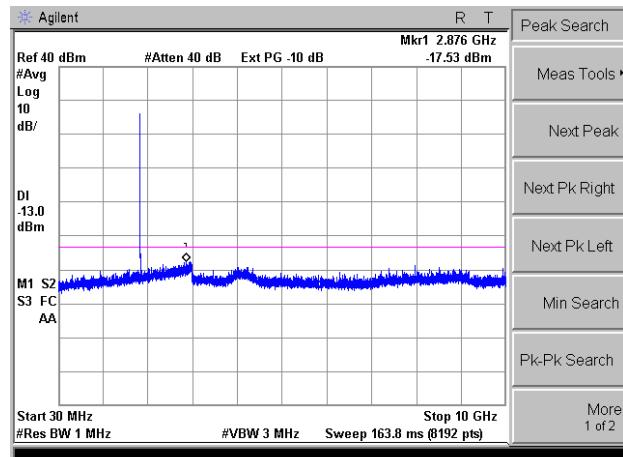
Conducted Emission Transmitting Mode CH 128
