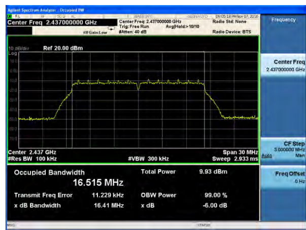
(802.11g) 6dB Bandwidth plot on channel 6
