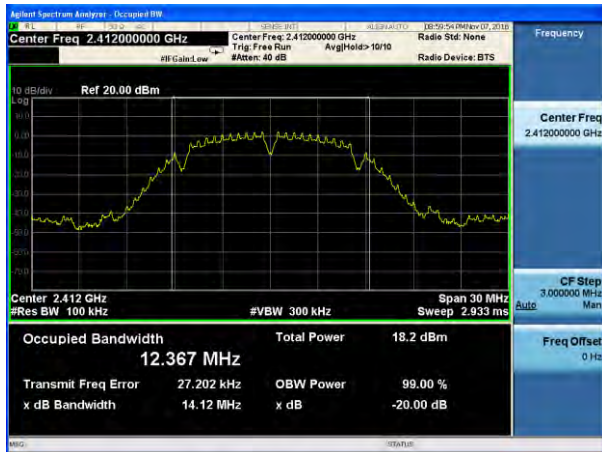
(802.11b) -20dB Bandwidth plot on channel 6
