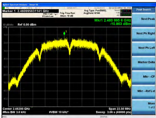
(802.11b) PSD plot on channel 11
