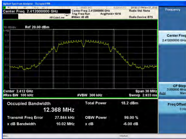
(802.11b) 6dB Bandwidth plot on channel 6
