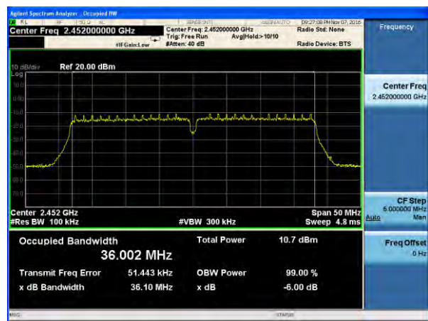
(802.11n40) 6dB Bandwidth plot on channel 9
