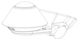
1. Use a coin to loosen the Dock hinge by turning the adjustment slot counter-clockwise.
