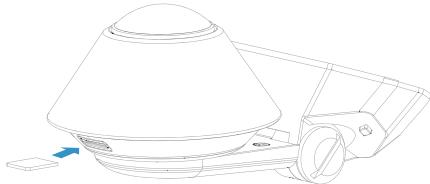
Waylens recommends using a high endurance microSD card (class 10 or higher MLC microSD card 32-256GB) designed for continuous recording situations. While other cards will work with the Secure360, they are much more prone to card errors and failures.
