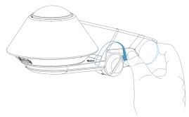
3. Tighten the Dock into place by turning the adjustment slot clockwise with a coin.
