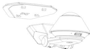
1. With the Mount Plate attached to the windshield and the power cord connected to the Secure360, position the Secure360 onto the Mount Plate.
