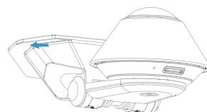
2. Slide the Dock left to secure it firmly on the Mount Plate.
