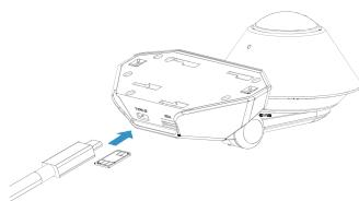
2. Turn on the vehicle accessory power or start the engine. The status LED will illuminate white (and turn red then if a SD card is inserted).
