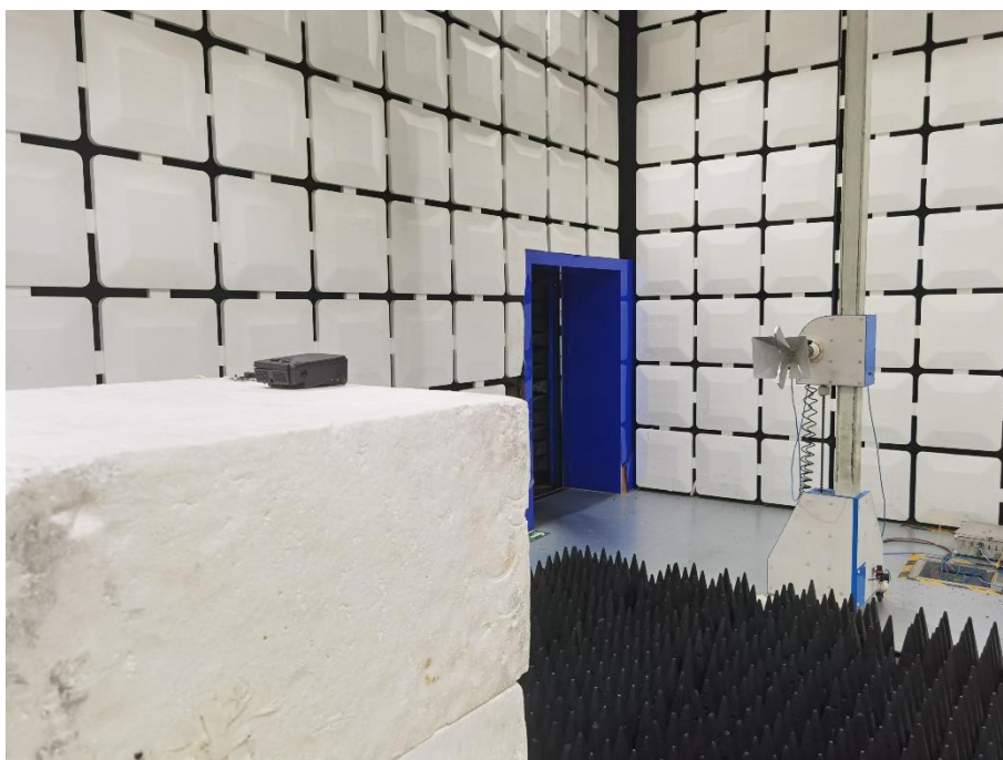
Description:RF Radiated Emission Test Setup for 1GHz ~ 18GHz (Mode1)
