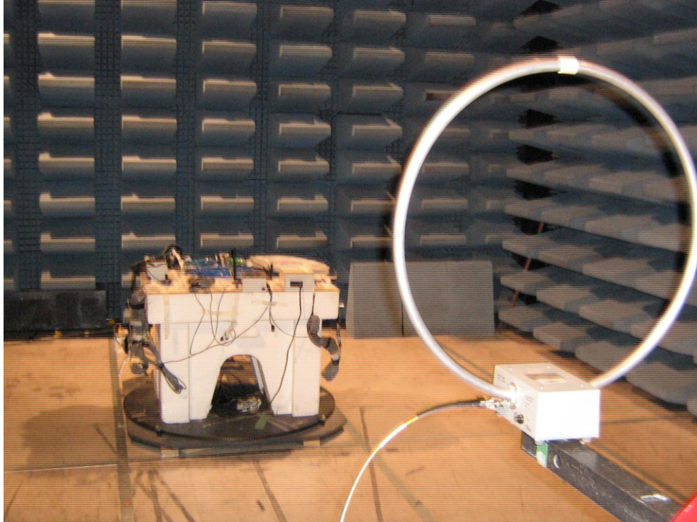
Figure 1: Radiated Emissions (below 30MHz) Test Setup
