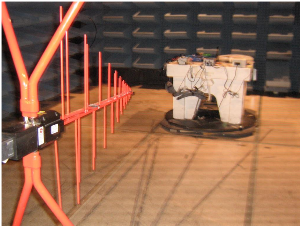
Figure 2: Radiated Emissions ( 30MHz – 1 GHz) Test Setup
