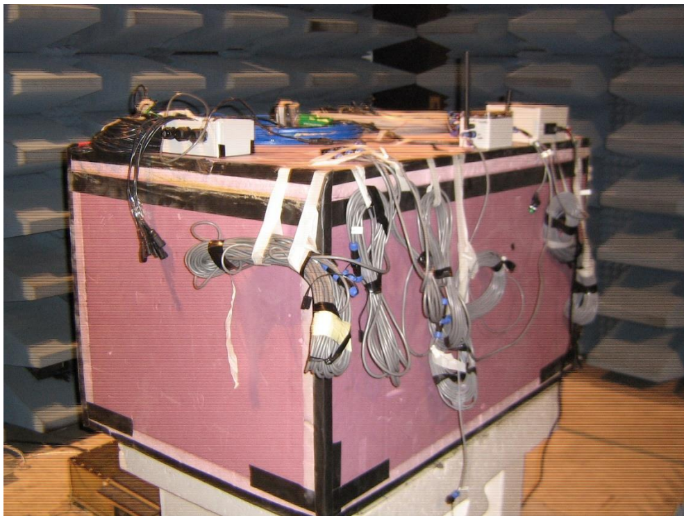
Figure 4: Radiated Emissions (above 1GHz close-up view) Test Setup
