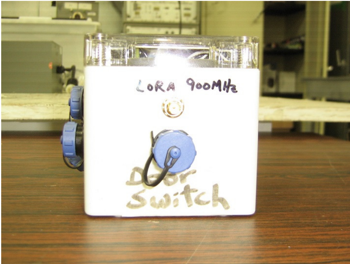
Side view of Transmitter exterior; note the antenna connectors are RPSMA(F)
