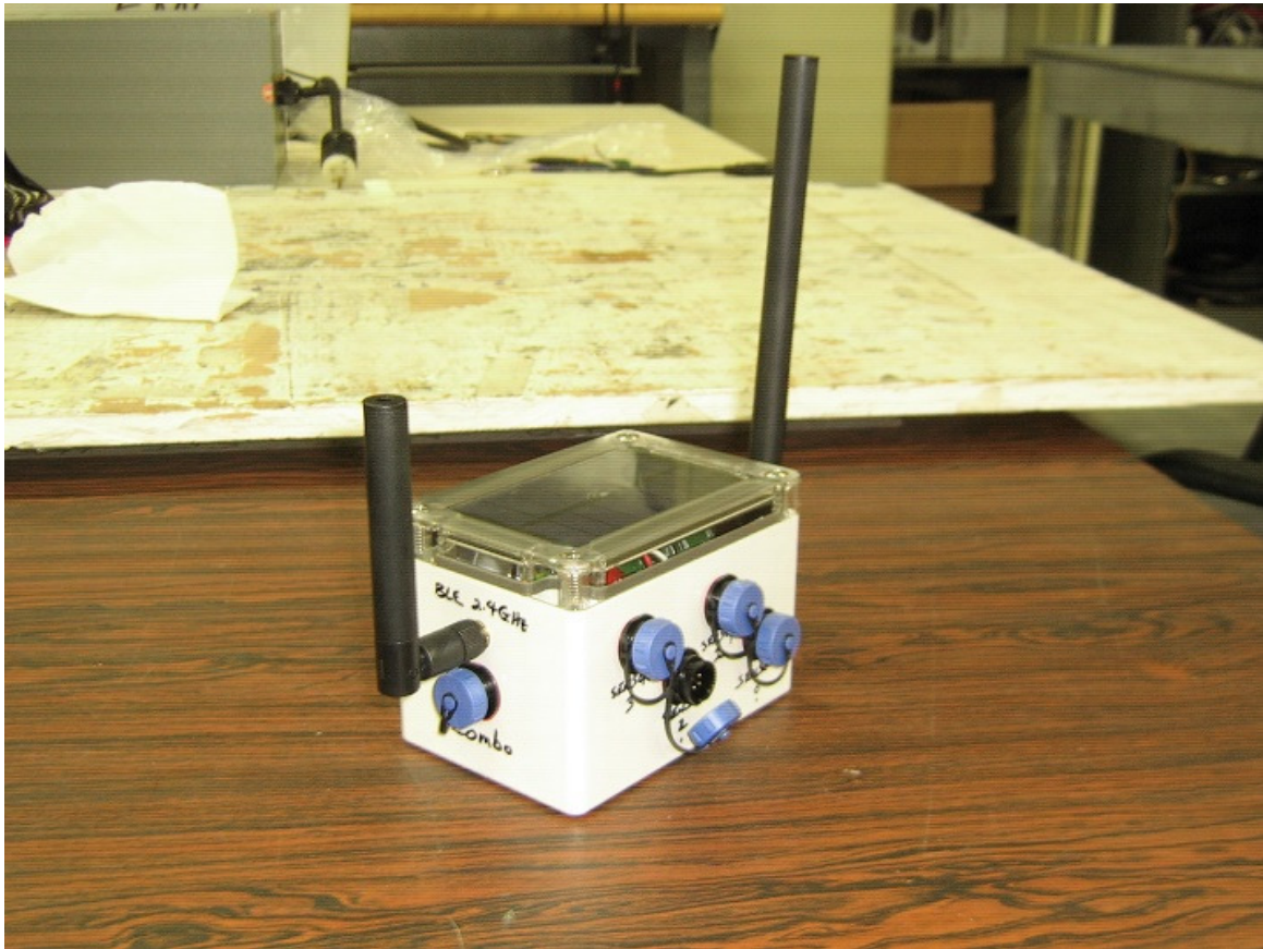
Complete Transmitter device with standard/default antennas installed
