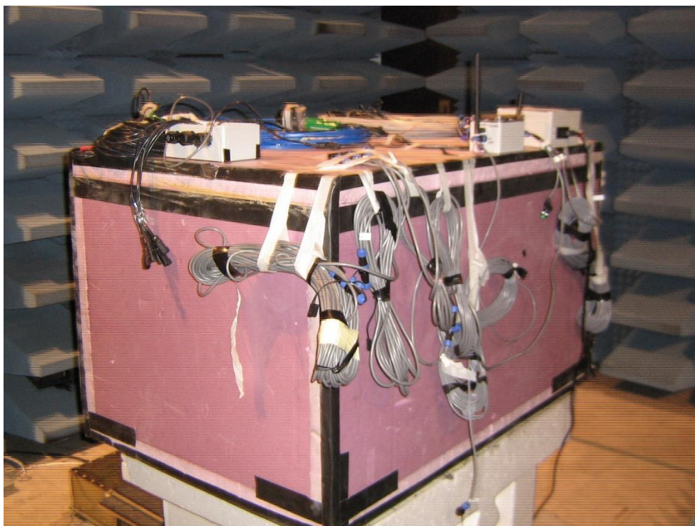
Figure 2: Radiated Emissions (above 1GHz close-up view) Test Setup
